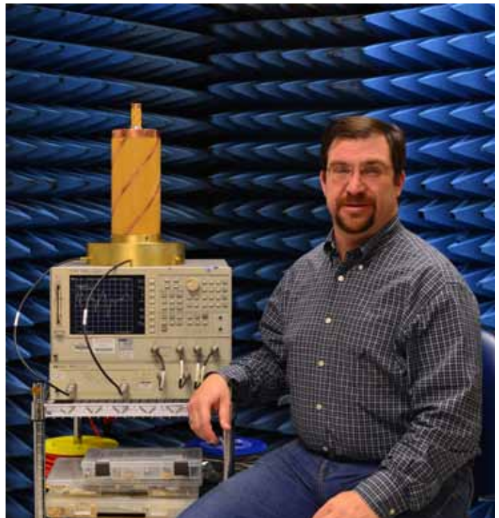
Nestor Voronka is helping to develop the cylindrical antenna shown connected to a network analyzer for a space-weather mission.
