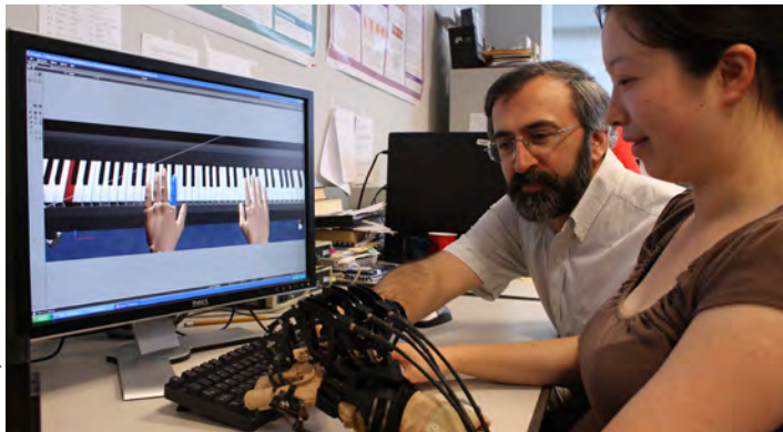
Associate Professor Sergei Adamovich and graduate student Qinyin Qiu working with a CyberGrasp Glove and virtual piano program designed to help stroke patients regain the use of hands and fingers.
