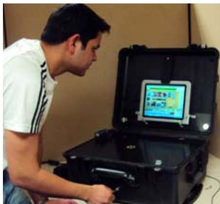
Parag Bargaonkar, AC Birox technical director, demonstrates how a sample is introduced into the ACB2000 for heating and vaporization prior to the gas chromatography stage.
